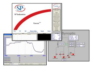
The Encore Control System is designed to meet the lyophilization requirements of pharmaceutical and biotechnology companies. The system utilizes the GE Fanuc Proficy® HMI/SCADA – iFIX solution for Windows and an Allen-Bradley MicroLogix 1500 Programmable Logic Controller (PLC). The software system meets Current Good Manufacturing Practice (cGMP) standards and regulatory guidelines for computer systems used for pharmaceutical processing equipment.
